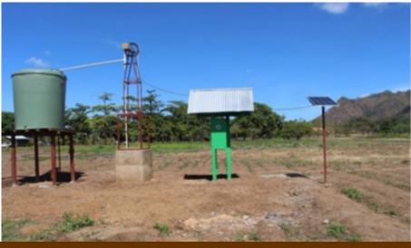
Solar Powered Rope and Washer Pump Technology Demonstration
